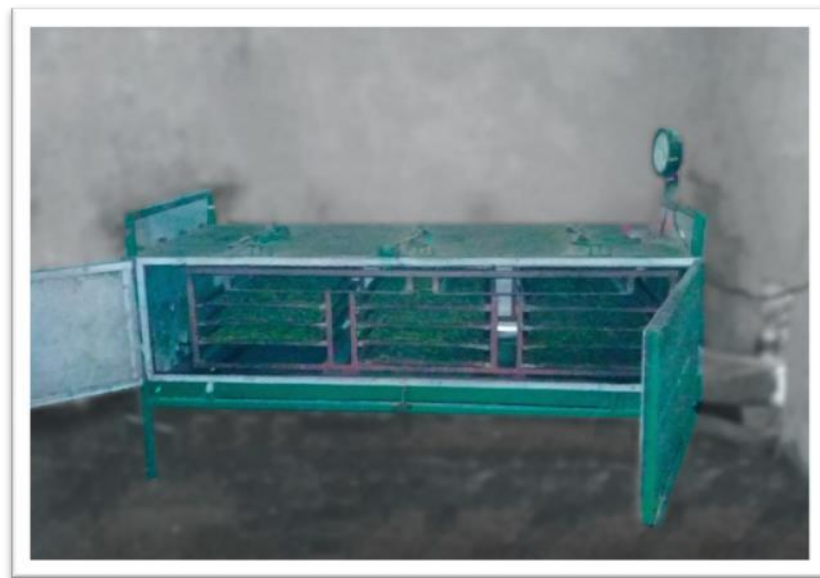
Reciprocating Tea Dryer Drying tray arrangement
