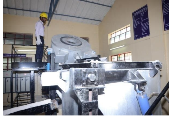
Melting and refining of aluminum scraps
