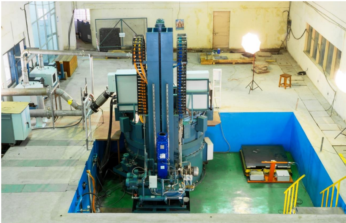
Fig. 2: Rotor Test Rig and Movable Pneumatic Loading Station in Pit
