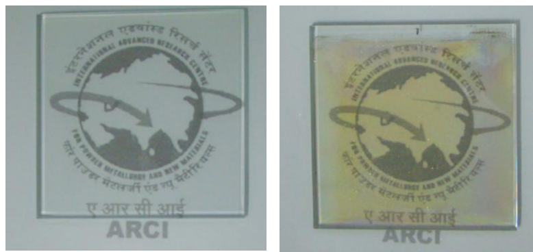
Fig 2 Photographs of uncoated (top) and solar control coated SLG substrate (10 cm x 10 cm) giving an idea of the visible light transmittance.
