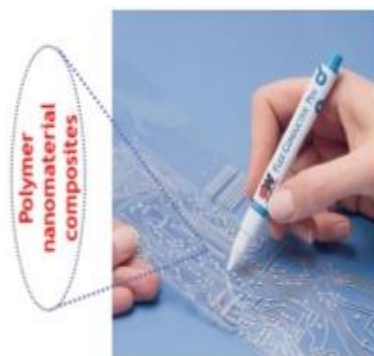
Figure: conductive polymer-nanomaterial composite patterned on a flexible substrate (https://www.chemtronics.com/circuitworks-conductive-pens-and-inks).
