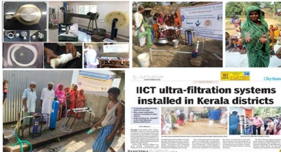
Prototype-2: Development of hand pump operated hollow fiber Ultrafiltration membrane systems for disaster management
