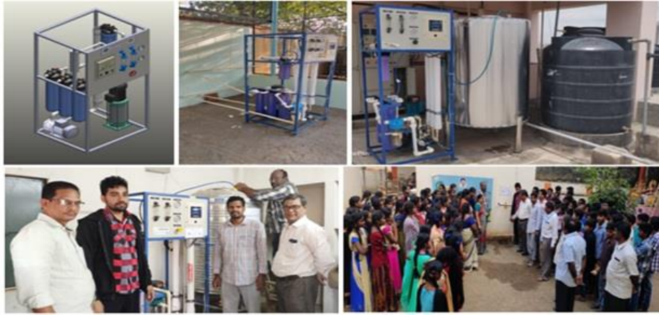
Prototype-1: Design of highly compact, vertical modular Nanofiltration membrane systems for removal of heavy metals from groundwater
