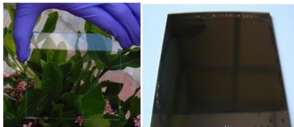
Antireflective coating on PV cover glass and Silicon wafer
