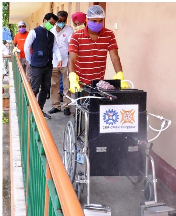
The sprayer systems in both BPDS and POMID are designed with two-stage spraying units and separate storage tanks to clean and disinfect the indoor areas by the numbers of fixed and flexible nozzles set in the lower and upper tiers. There is also an industrial variant of the Disinfectant Sprayer for heavy usage and to cover a larger area.
