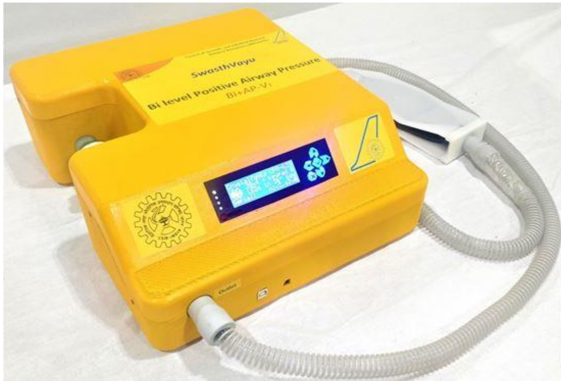
SwasthVayu BiPAP machine in Auto Test mode with Test Lung
