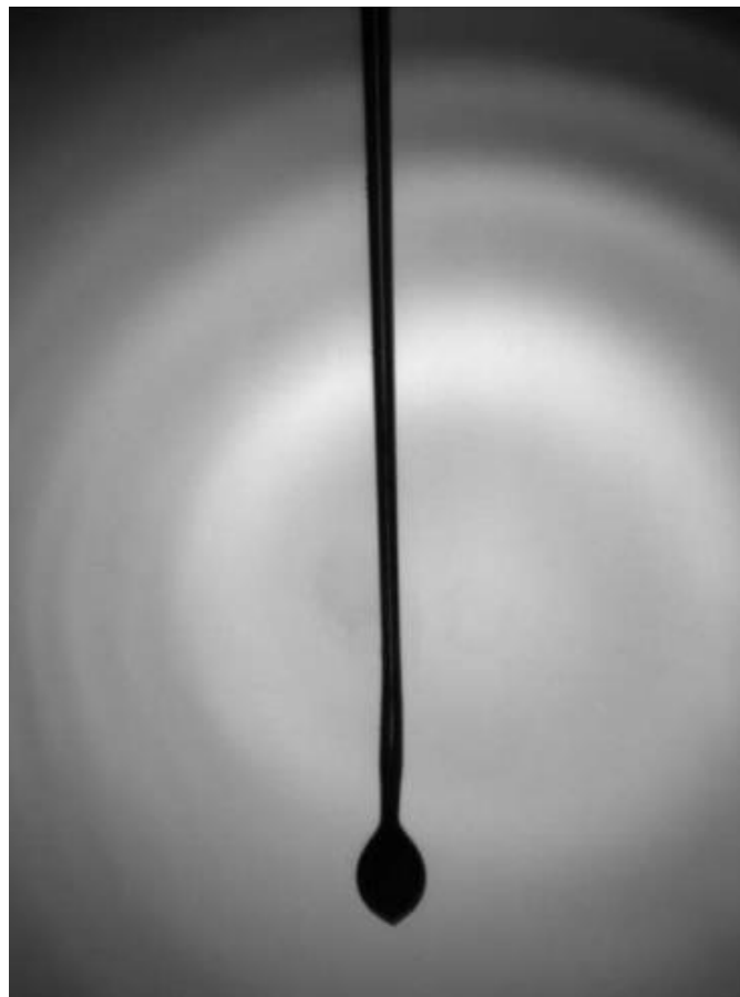
Image from toluene droplet combustion process (Photo: Sankaranarayanan et al.)
