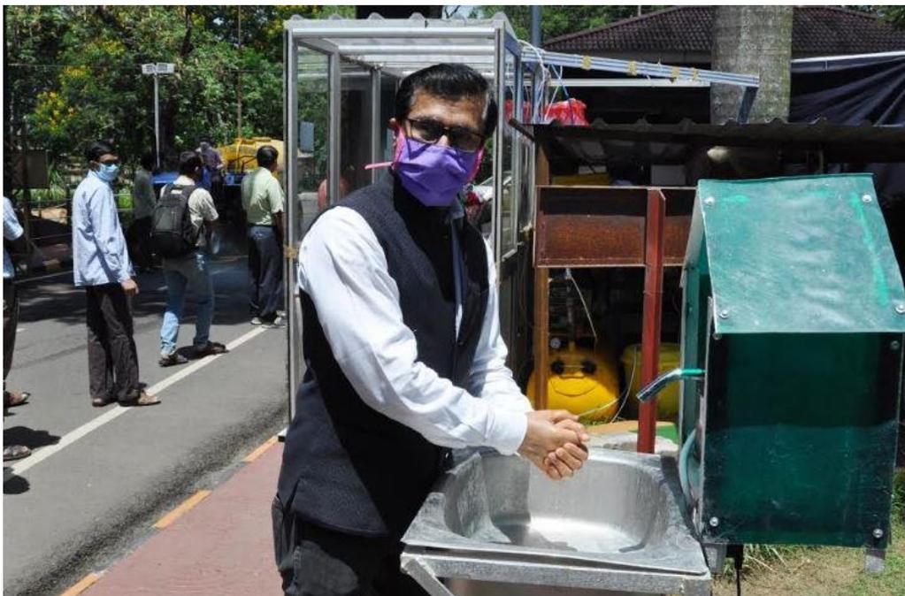
The single infrared sensor attached to the dispensing unit gets automatically activated when an object comes close to the unit. Other important design features of this unit include dispensing of both liquid soaps and water from the same outlet 20 seconds apart. The touch-less soap-cum-water dispensing units may find their utility at various locations such as hospitals, shopping malls, banks, stadiums, and sports complexes.
