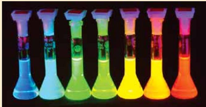
Fig. 2 : Fluorescence in different-sized CdSe quantum-dots
