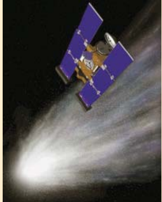
The Stardust spacecraft collected dust from the tail of Comet Wild-2 and brought it back to Earth for analysis
