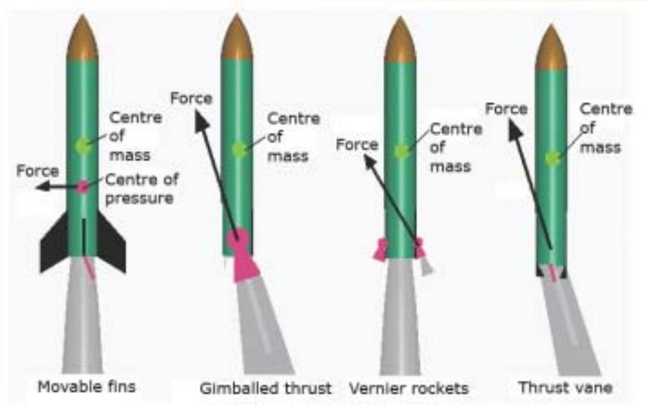
Fig. 4. Different methods of rocket control
