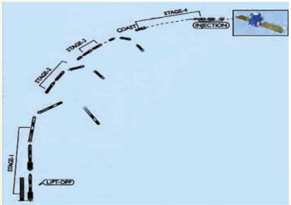
Fig. 3. Path of a multistage rocket
