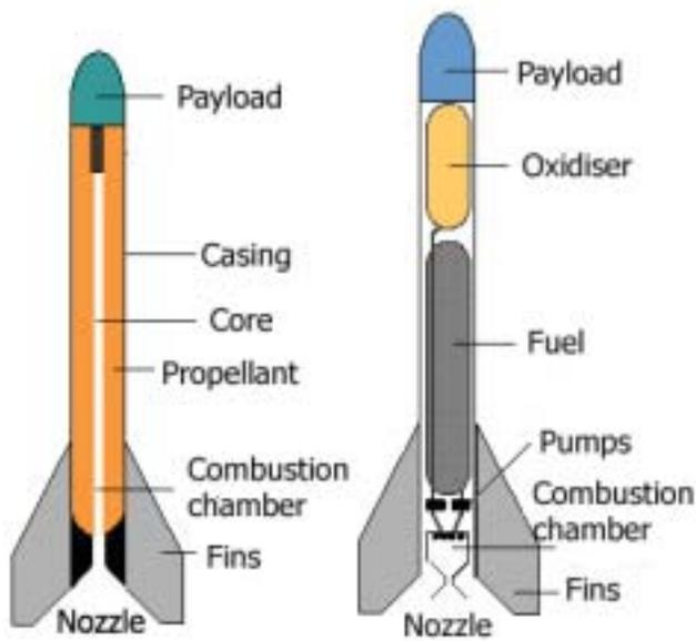
Fig. 2. Solid (left) and liquid propellant (right) rockets
