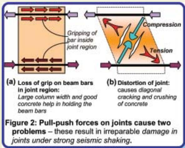
Further, under the action of the above pull-push forces at top and bottom ends, joints undergo geometric distortion; one diagonal length of the joint elongates and the other compresses (Figure 2b). If the column cross-sectional size is insufficient, the concrete in the joint develops diagonal cracks.
