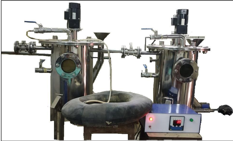
Laboratory scale anaerobic reactor - 45 litre capacity
