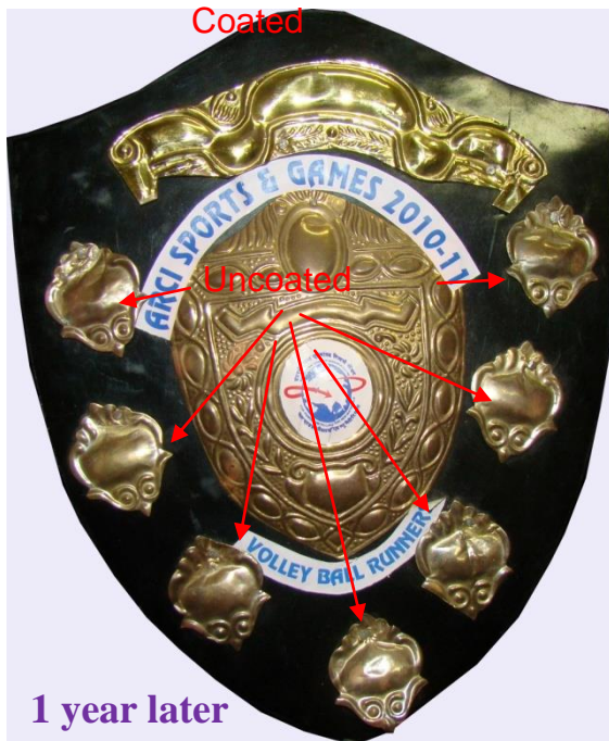
Perspiration resistance test on coated and uncoated silver substrates
