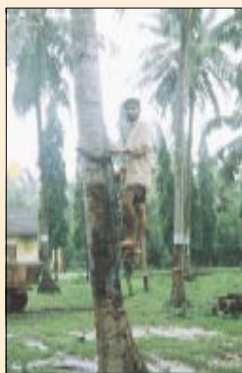
An equipment to climb up a coconut tree developed at the station.
