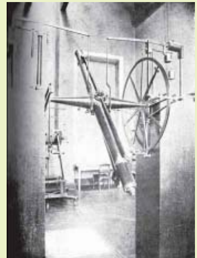
Gauss' principal instrument, the Repsold meridian circle
