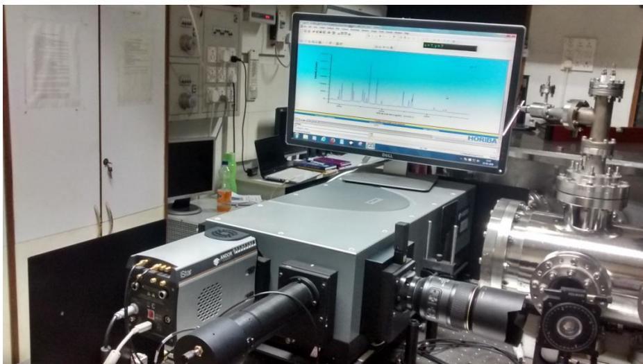
The newly acquired ICCD spectrometer from Andor Technology Ltd, UK, has augmented the laser plasma measurement capabilities of the lab
