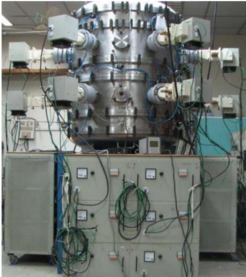
Large Volume Plasma System using multiple Compact ECR Plasma Sources
