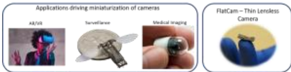
Figure 1. Left – Applications that require miniature cameras. Right – FlatCam - an ultra-thin lensless camera developed by Rice University, USA.
