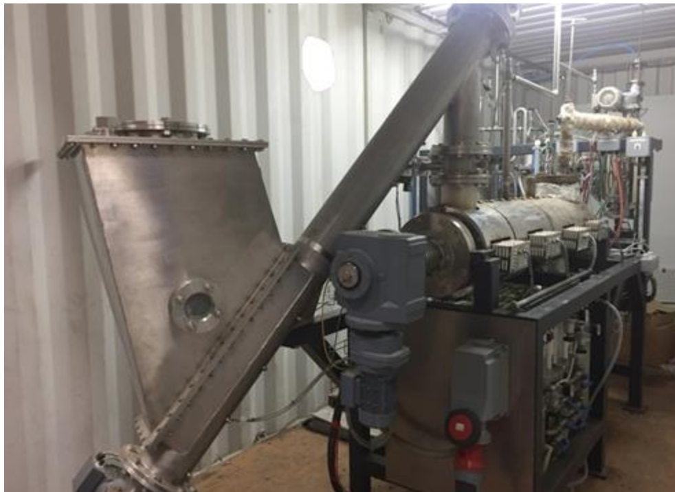
E-waste Pyrolysis Pilot Plant (10 kg/h)
