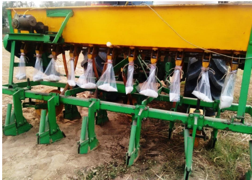
Fertilizer dropped is collected into zipper bags during operation
