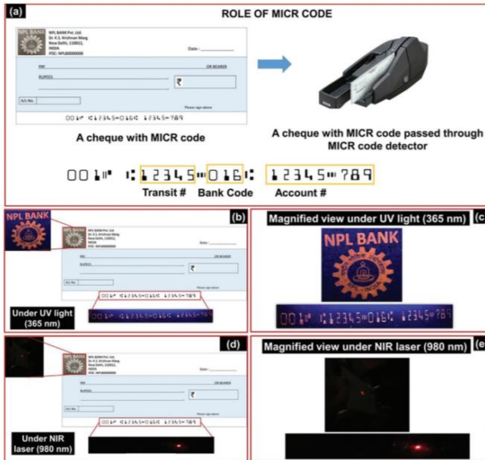
Figure 4. a) schematic for the explanation of role of MICR code on hypothetically proposed bank name and cheque, how it has been detected and the information it carries by demonstrating the sample cheque printed in the lab using multi-functional security ink; optical images of features present on sample cheque b) under UV light (365 nm); c) its magnified view; d) under NIR laser (980 nm); and e) its magnified view.
